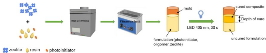
Figure 1. Preparation of zeolite/polymer composites via photopolymerization.
