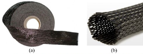
Fig. 2. The braided fabrics, (a) a flat fabric and (b) a tubular fabric
